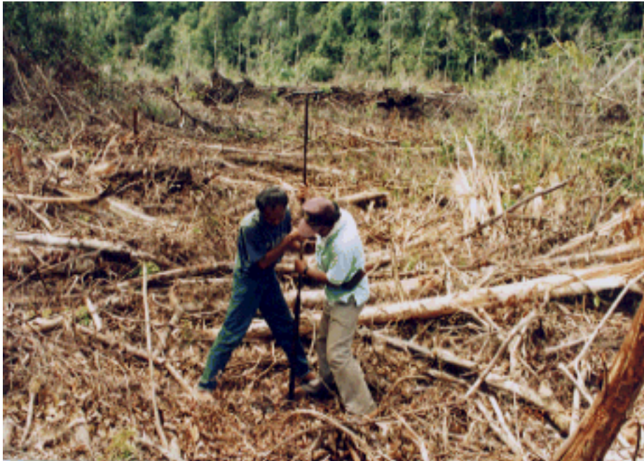
Figure D.7. Staffs are boring peatland to explore the depth and type of peatland at central Borneo, August 1996.
